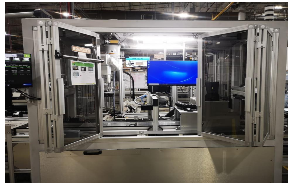
Tester integration for inspection, electrical test and laser marking (KEYENCE laser marking machine)
