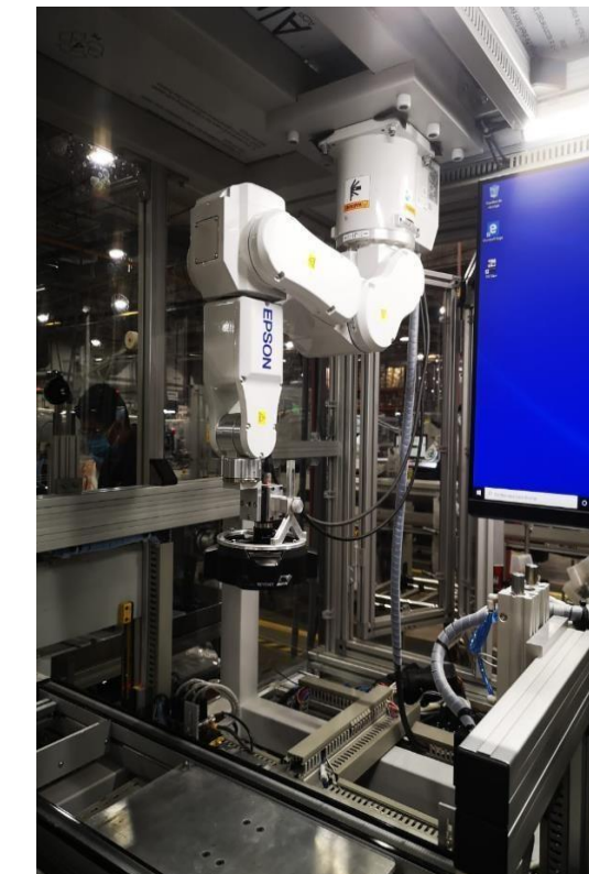
Integration of EPSON robot with KEYENCE Vision System
